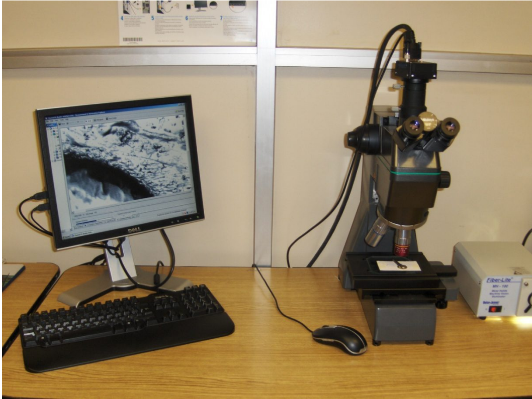
Figure 5. Optical microscope system, CCD camera, and computer. The sample is a metallic key.
