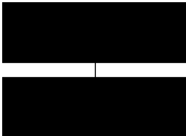
Figure 10. Filter transfer function H(u, v) . It suppresses the low frequencies and high frequencies related with horizontal direction by means a and b parameters.
