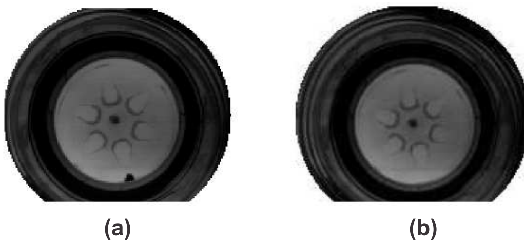
Figure 8. Bottle bottom (a) with defect and (b) without defect.
