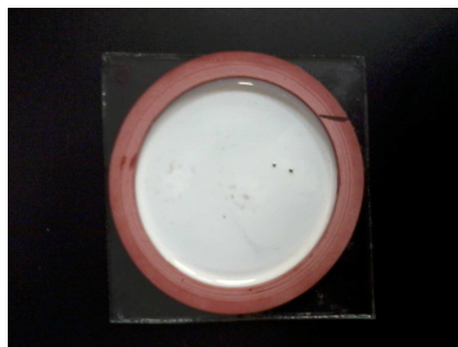
Figure 1. Image of a phantom tissue prepared with a polyurethane varnish base and catalyst for polyurethane varnish in equal portions, titanium dioxide particles (TiO 2 ) and coffee particles to simulate a skin lesion.
