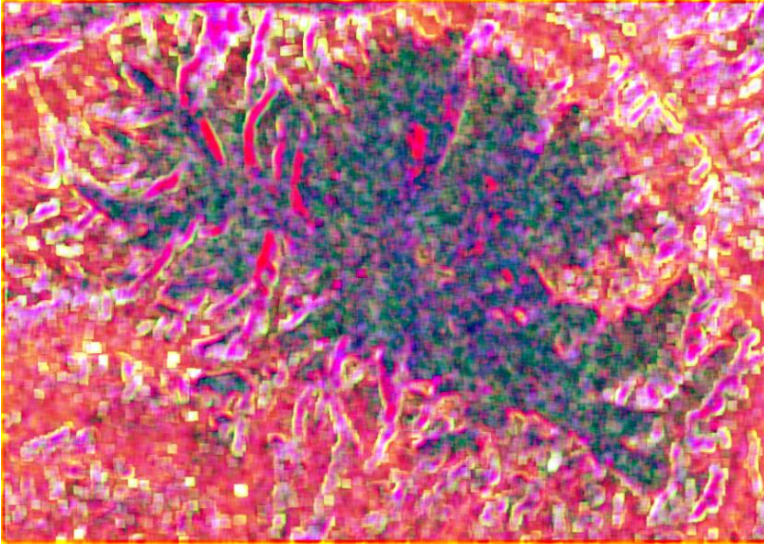
Figure 3. A colour image created by the texture filters (R=result of the contrast filter, G=result of the correlation filter, B=result of the skewness filter).
