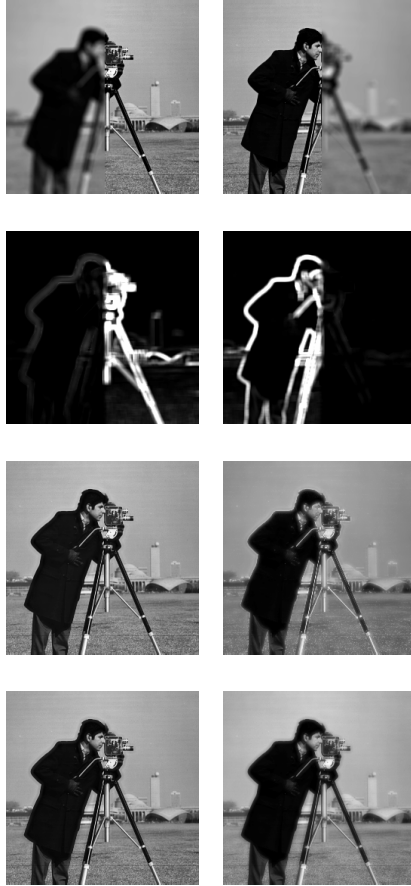
Figure 1. Case 1. Top: input images x_A (left) and x_B (right). Second row: total weights c \cdot \lambda (left) and c \cdot (1 - \lambda) (right). Third row: fused images with a Laplacian (left) and a ratio (right) pyramid decompositions. Bottom: fused images with a SIDWT (left) decomposition and averaging (right).
