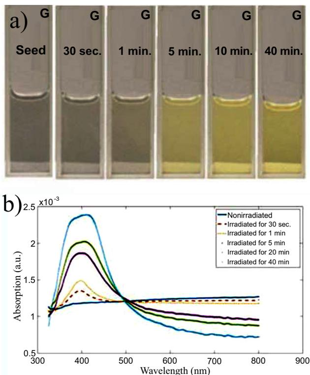
**Fig. (3).** a) Photographs of AgNPs suspended in ethanol before (seed) and after laser light irradiation with an energy of  $60 \mu\text{J}$  for 30 seconds, 1, 5, 10 and 40 minutes, respectively. b) Absorption spectra of the colloidal solutions.
