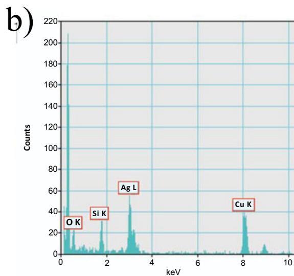
**Fig. (5).** a) AgNPs generated with a laser energy of  $60 \mu\text{J}$  for 10 minutes. b) EDS analysis.
