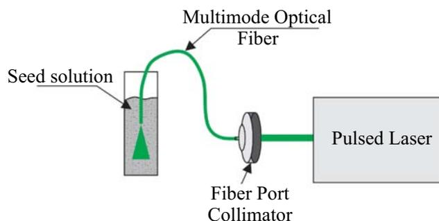
Fig. (1). Experimental setup to obtain silver colloidal solution.
