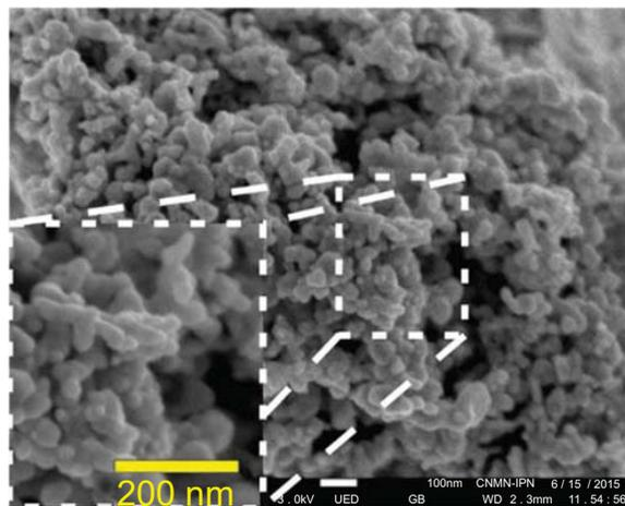
Fig. (2). SEM micrographs of silver nanopowder.
