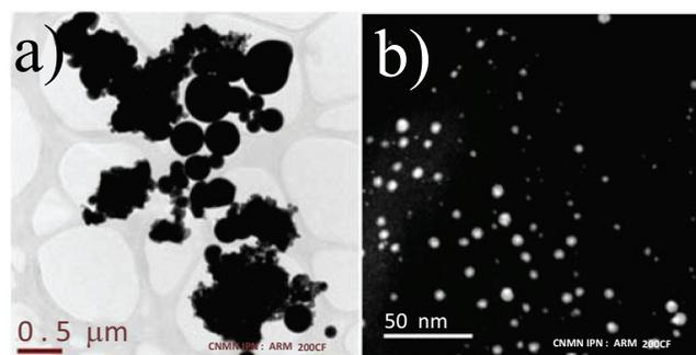
**Fig. (4).** TEM micrographs of AgNPs obtained by: a) irradiating the seed solution for 40 minutes with a laser energy of  $60 \mu\text{J}$  and b) centrifuging the colloidal solution for 30 minutes with a rotation speed of 300 g.
