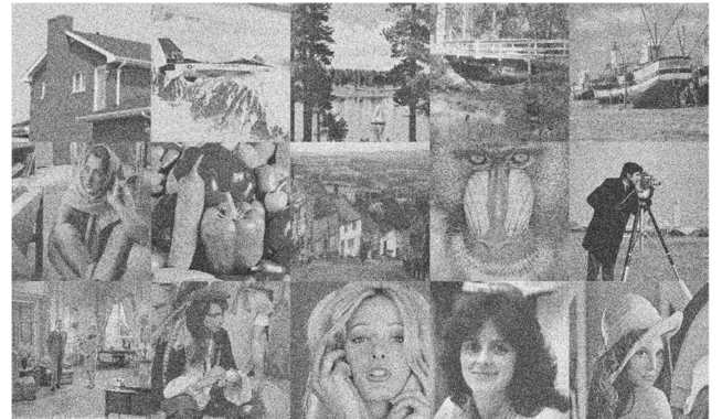
Fig. 10 15 standard test images corrupted by additive Gaussian noise of zero mean and \sigma^2 = 0.1
