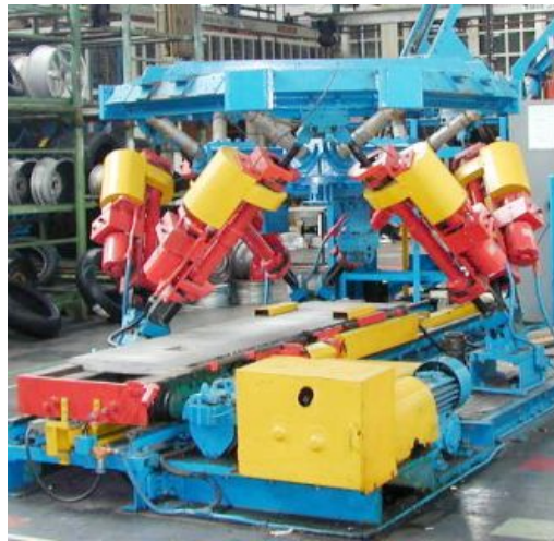
Figure 1.7: Gough Platform [Gough and Whitehall, 1962]
