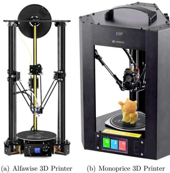
Figure 1.18: Examples of 3D printers based on PKMs
