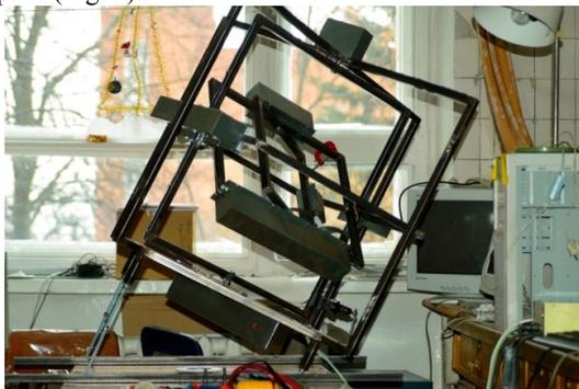
Fig. 5. Rotary device that points automatically the sources' beams to a fixed point in sky.
